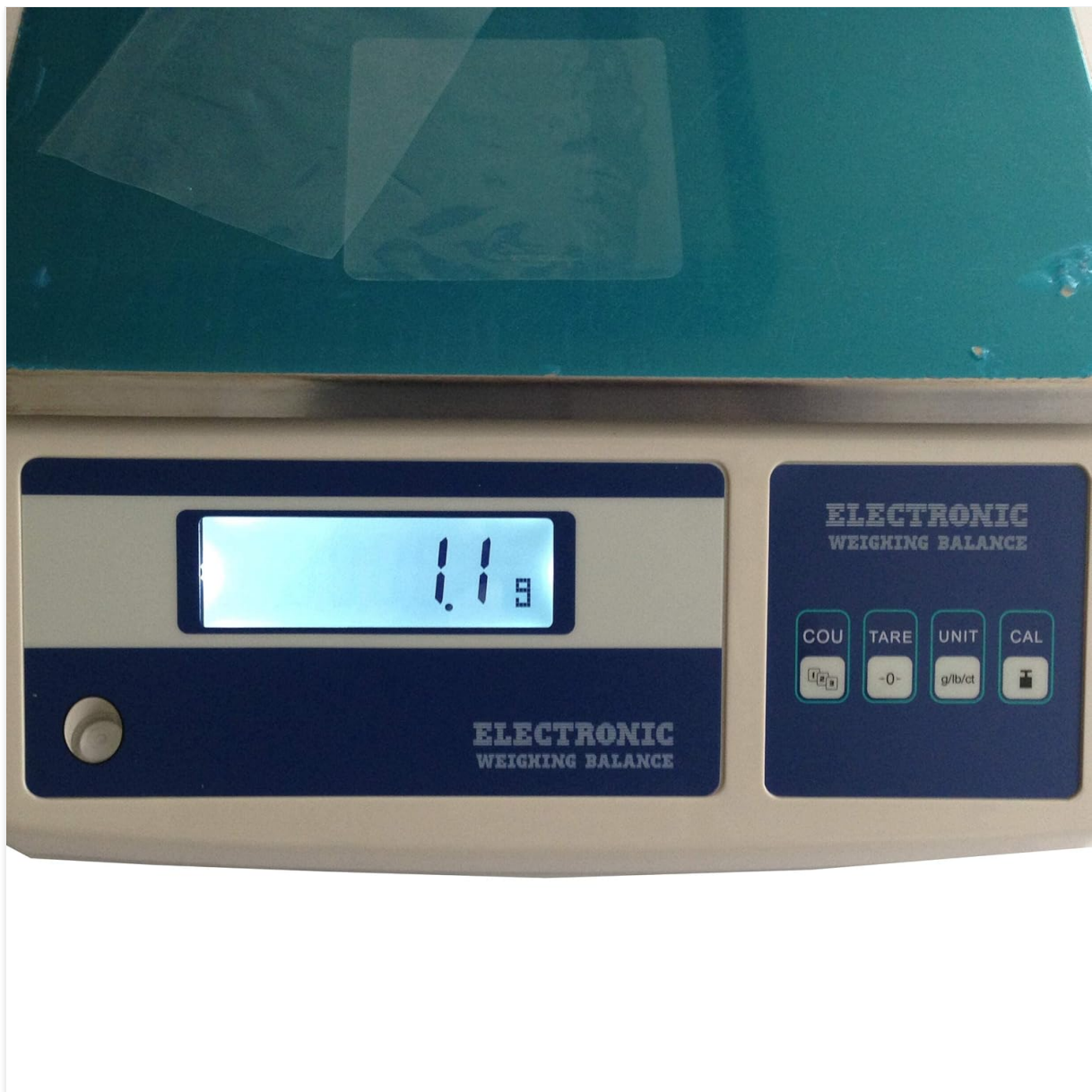
Figure 2: Close-up of the control panel, highlighting the 'COU' (Counting), 'TARE', 'UNIT', and 'CAL' (Calibration) buttons, alongside the digital LCD display.
