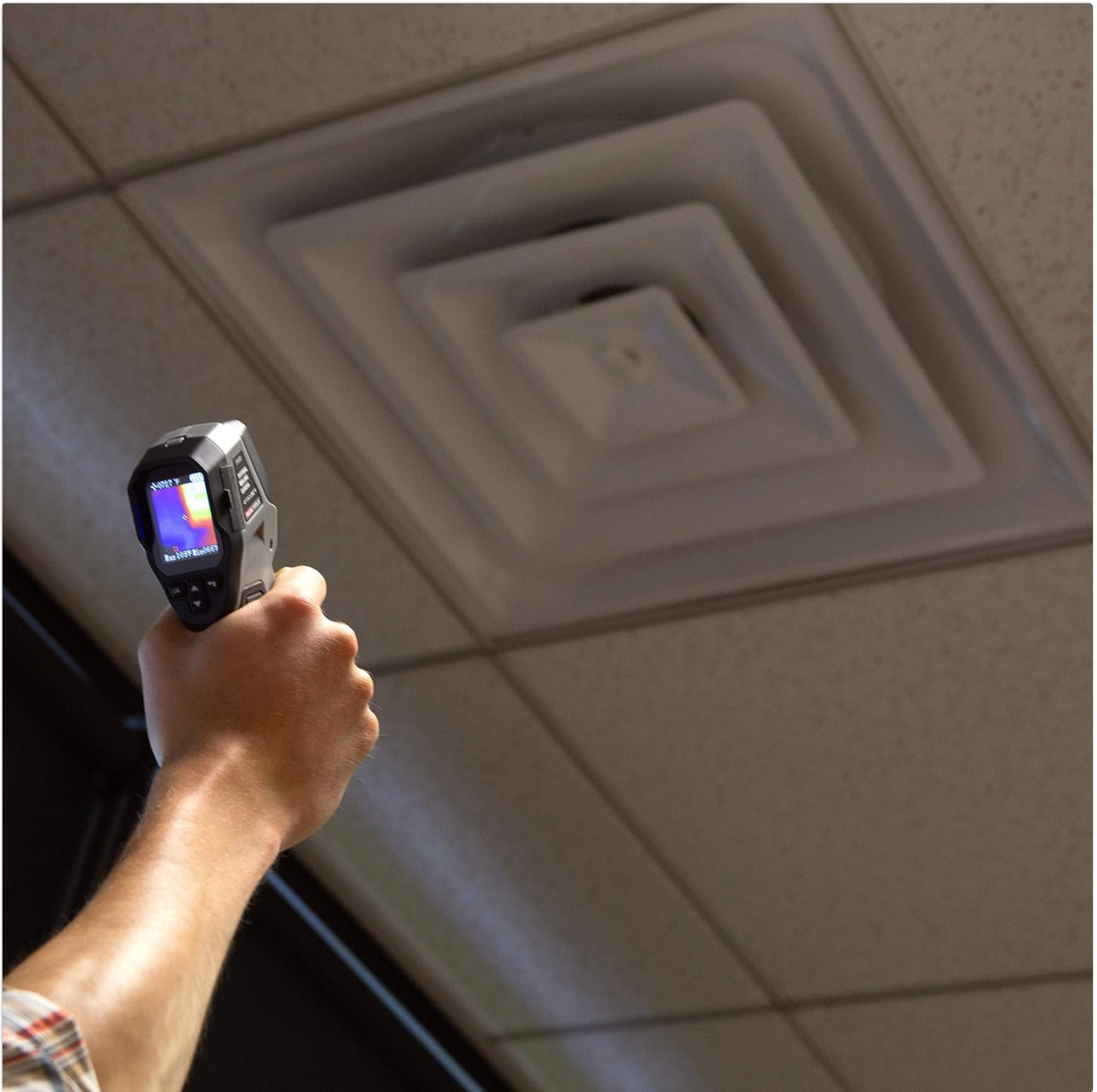
Image 6.3: Checking a ceiling vent for drafts or insulation deficiencies, helping to identify areas of heat loss or gain in a building.
