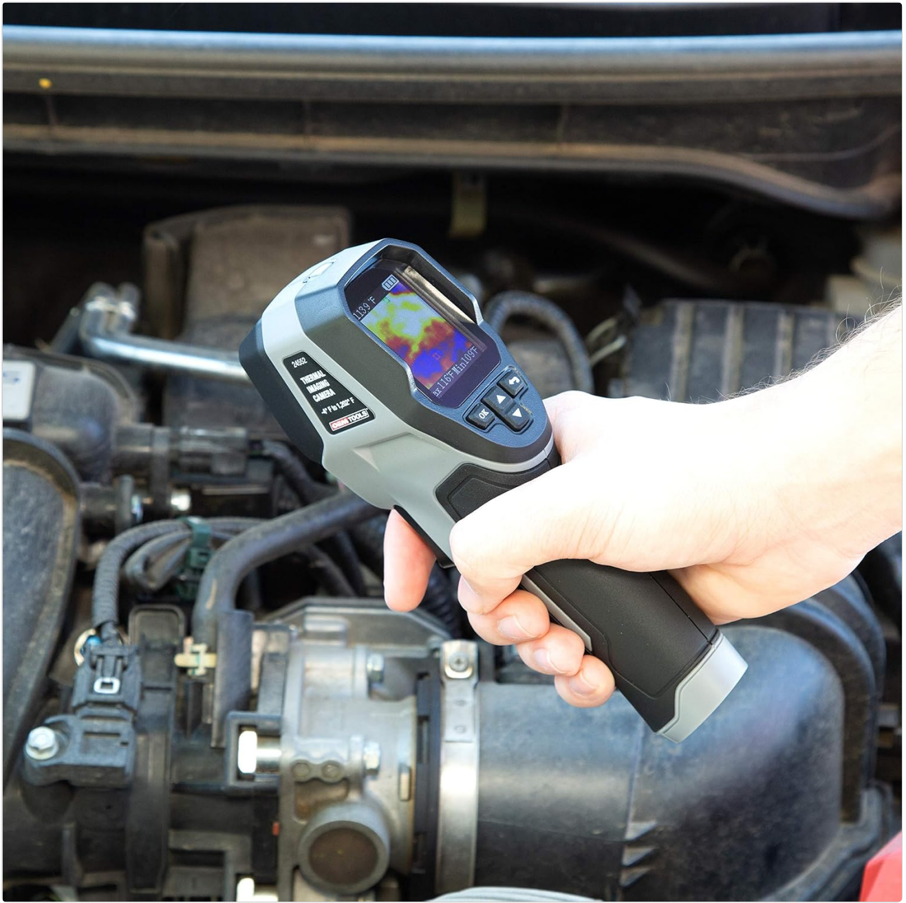
Image 6.2: Inspecting an engine bay for heat signatures, indicating potential issues like coolant leaks or overheating components.
