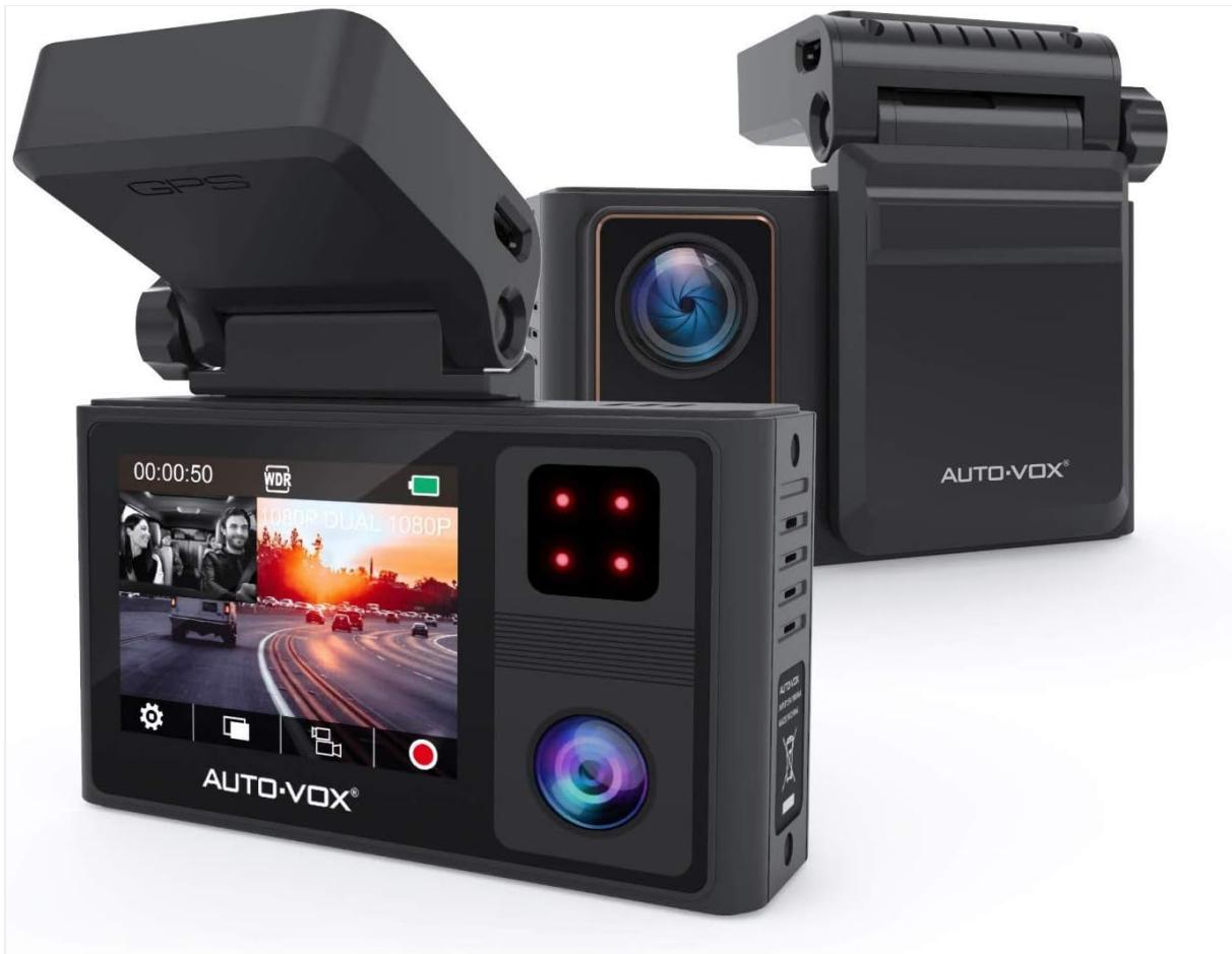
This image illustrates the dash cam's screen displaying a split view of both the front road and the vehicle's interior, confirming simultaneous dual recording capability.
