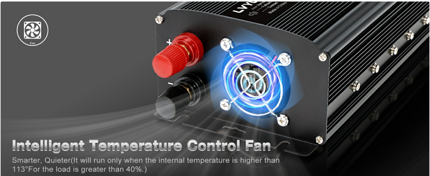
Image 4.1: The intelligent temperature control fan, which activates when the internal temperature exceeds 113°F or the load is greater than 40%, helping to maintain optimal operating temperature.
