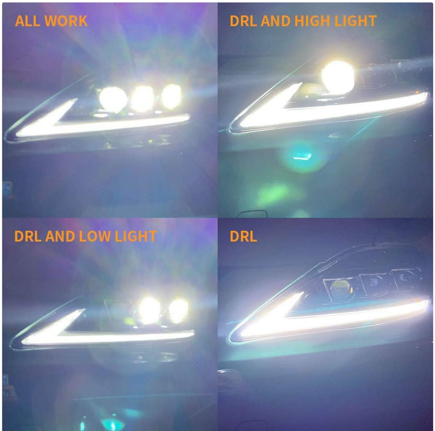
Image: A four-panel image displaying the headlight in different operational modes: all lights active, DRL with high beam, DRL with low beam, and DRL only, illustrating the various illumination patterns.
