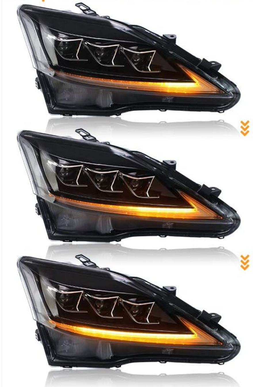
Image: A series of three images demonstrating the sequential illumination of the turn signal, showing the progressive lighting effect from the inner to the outer edge of the headlight.
