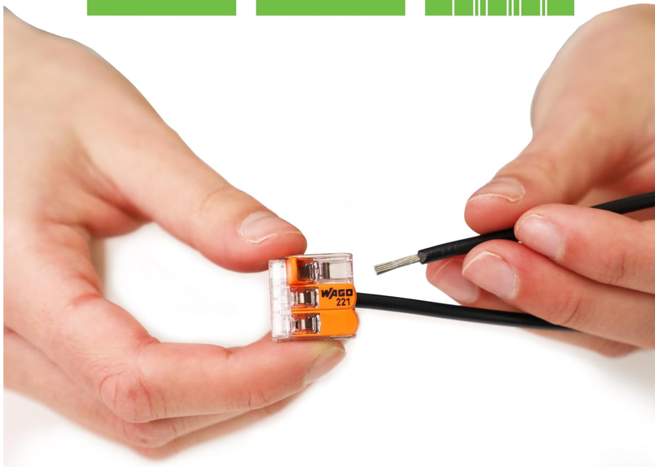
Figure 1: Wire Preparation. This image illustrates the correct wire stripping length (11 mm) required for optimal connection with the WAGO 221-413 Lever-Nuts connector. Proper stripping ensures full contact and secure termination.
