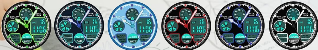
Image 4.1: Illustration of the watch display with and without the EL backlight activated.
