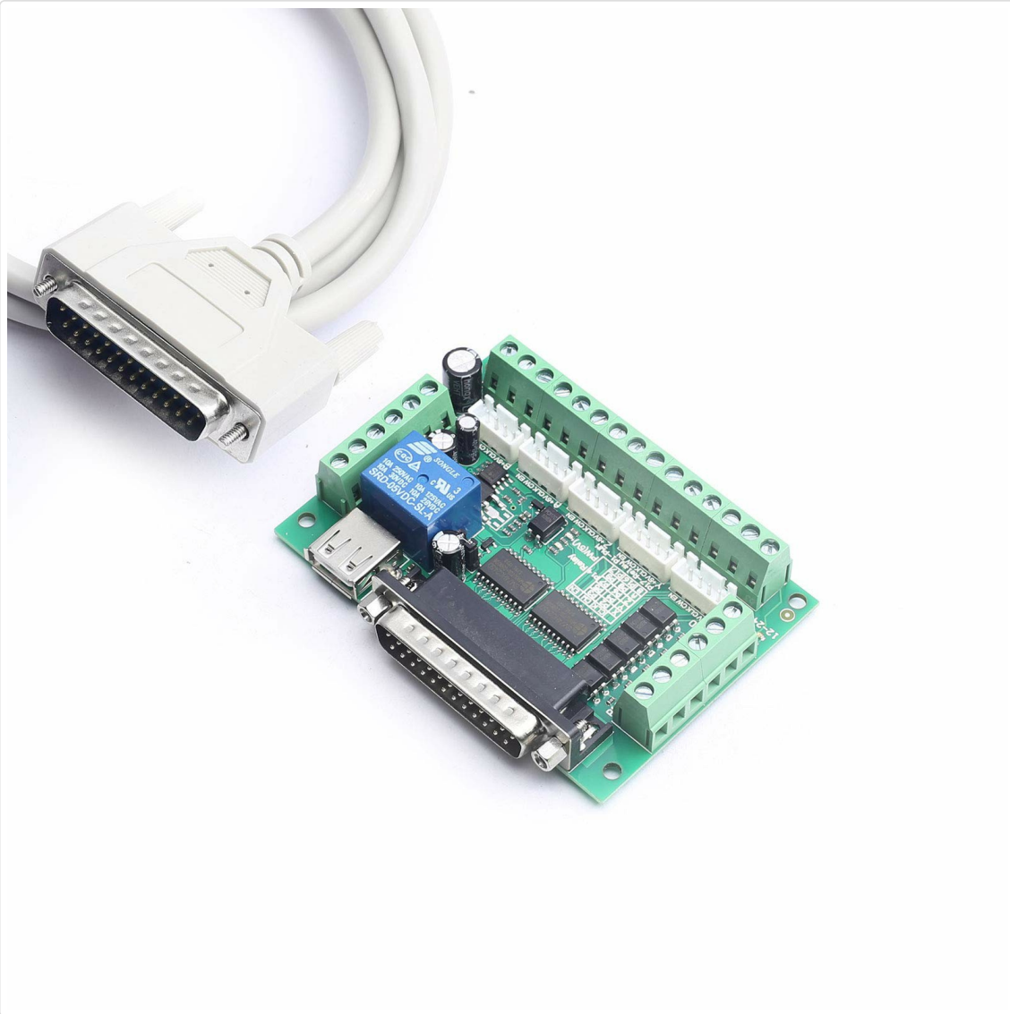
Figure 1: Top view of the DEVMO 5 Axis CNC Interface Adapter Breakout Board. This image shows the main components including the DB25 parallel port connector, USB power input, and terminal blocks for motor driver connections.
