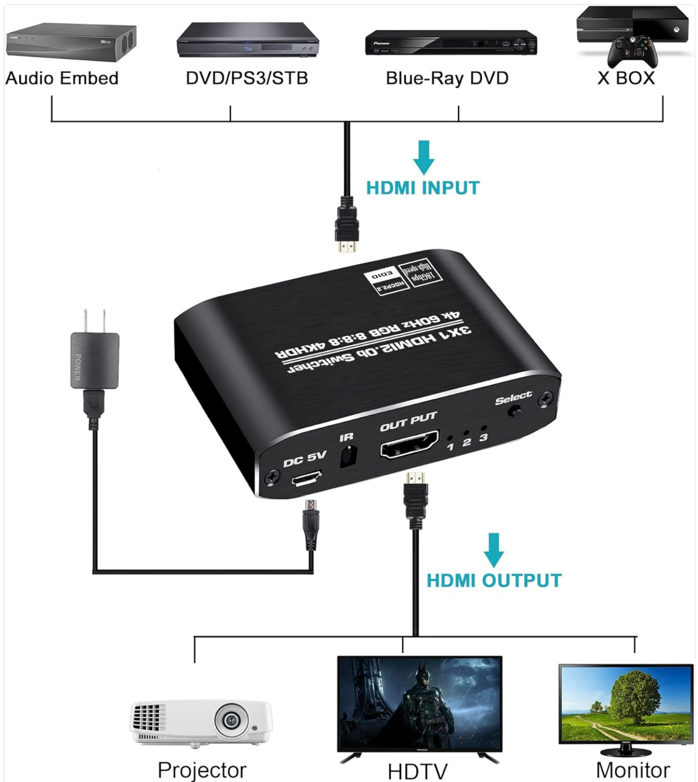
Image: Connection diagram illustrating how to connect various HDMI input devices (Audio Embed, DVD/PS3/STB, Blu-Ray DVD, XBOX) to the HDMI switch's input ports, and how the switch's output connects to a display (Projector, HDTV, Monitor), along with the power connection.
