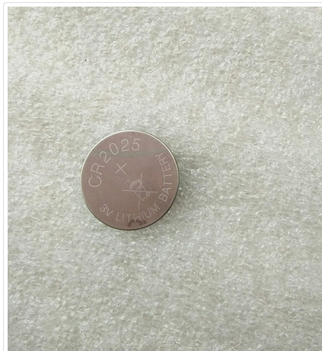
Figure 2: A CR2025 3V lithium coin cell battery, the required power source for the remote.
