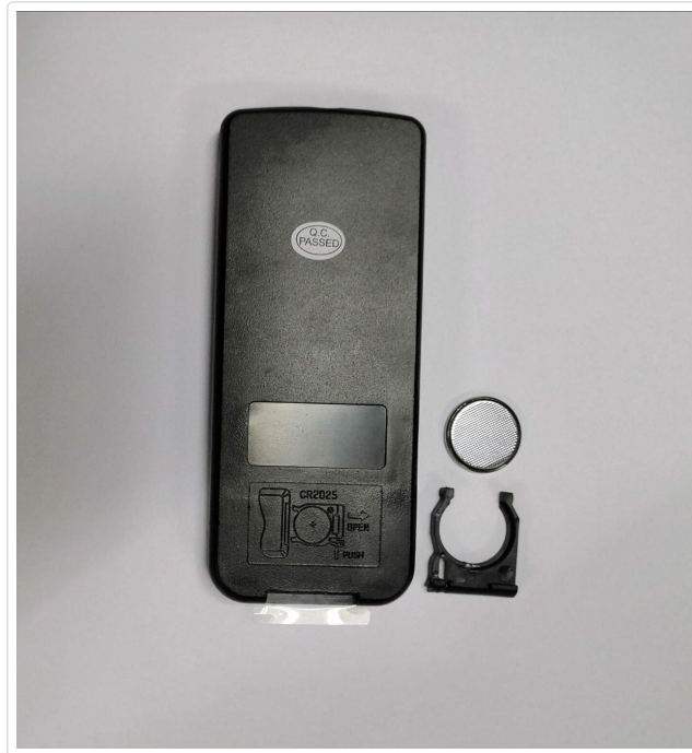
Figure 1: Back of the IRV-R2 remote control with the battery compartment open, illustrating the battery insertion method.
