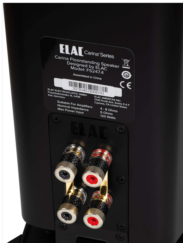
Image: Detailed view of the rear panel of the ELAC Carina FS247.4-SB speaker, showing the dual binding posts for amplifier connection.
