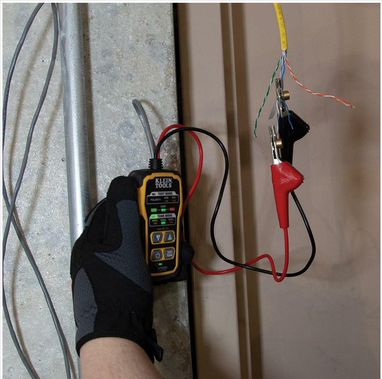
Image 4.1: The Toner-Pro connected to bare wires using the Angled Bed of Nails (ABN) clips.
