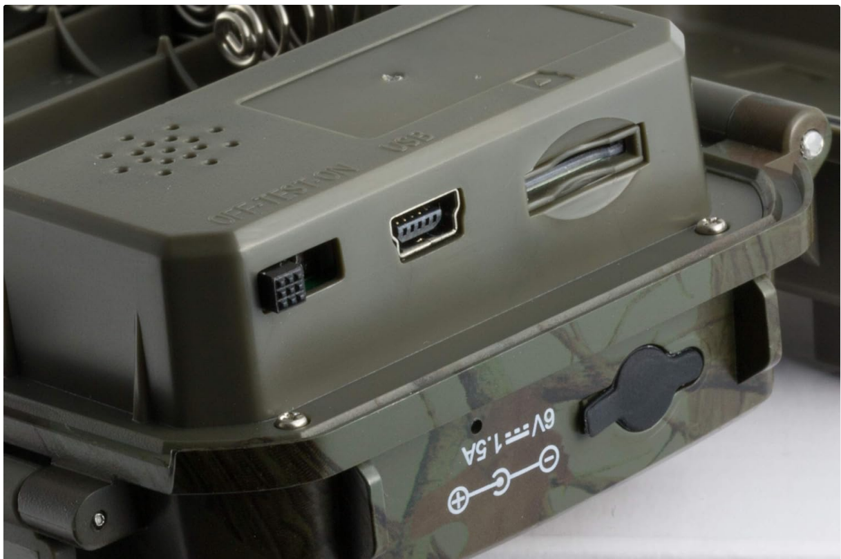
Figure 4: Bottom view of the camera, illustrating the external power input (6V/1.5A) and Mini USB port.
