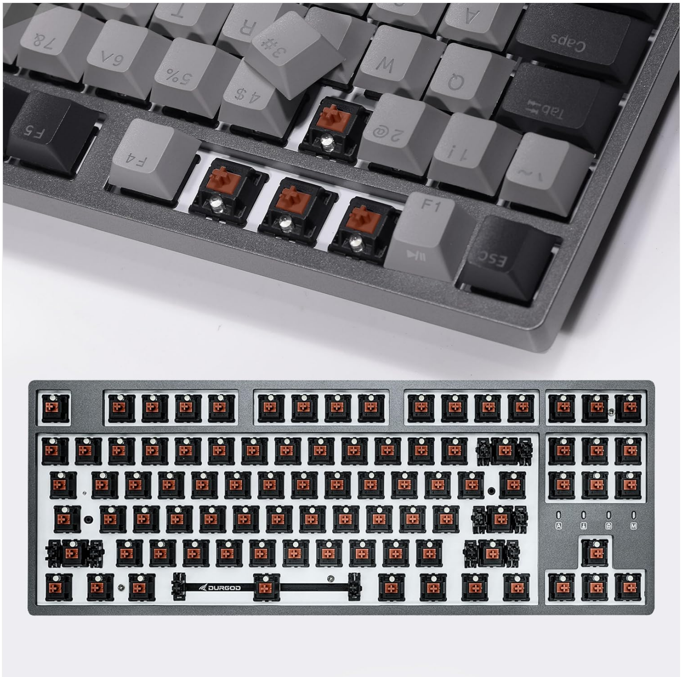
Image: A close-up view of the keyboard with some keycaps removed, revealing the Cherry MX switches underneath for cleaning.
