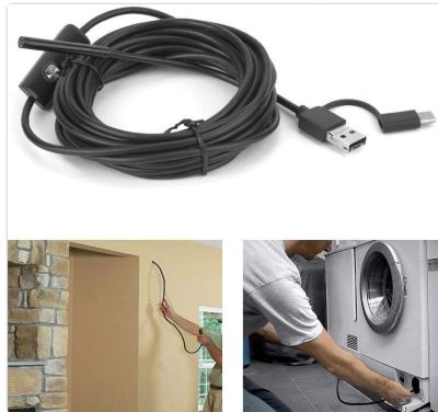
Figure 5: The 5-meter cable in a coiled state, showcasing the versatile 3-in-1 USB connector that includes standard USB-A, Micro-USB, and USB-C options.
