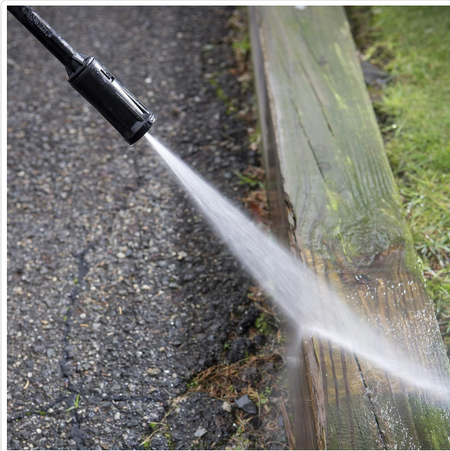
Figure 3: Demonstrating the pressure washer's effectiveness on a wooden surface, showing the concentrated spray removing grime.
