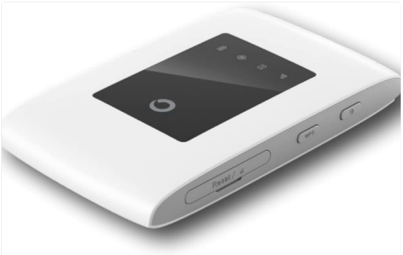
Figure 2: Angled view of the hotspot, highlighting the power button and the WPS (Wi-Fi Protected Setup) button on the side. A small reset pinhole is also visible.
