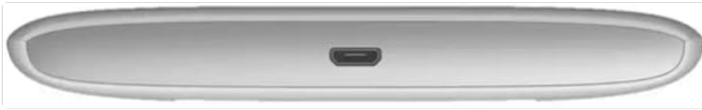
Figure 3: Bottom view of the device, showing the micro USB port used for charging the hotspot.
