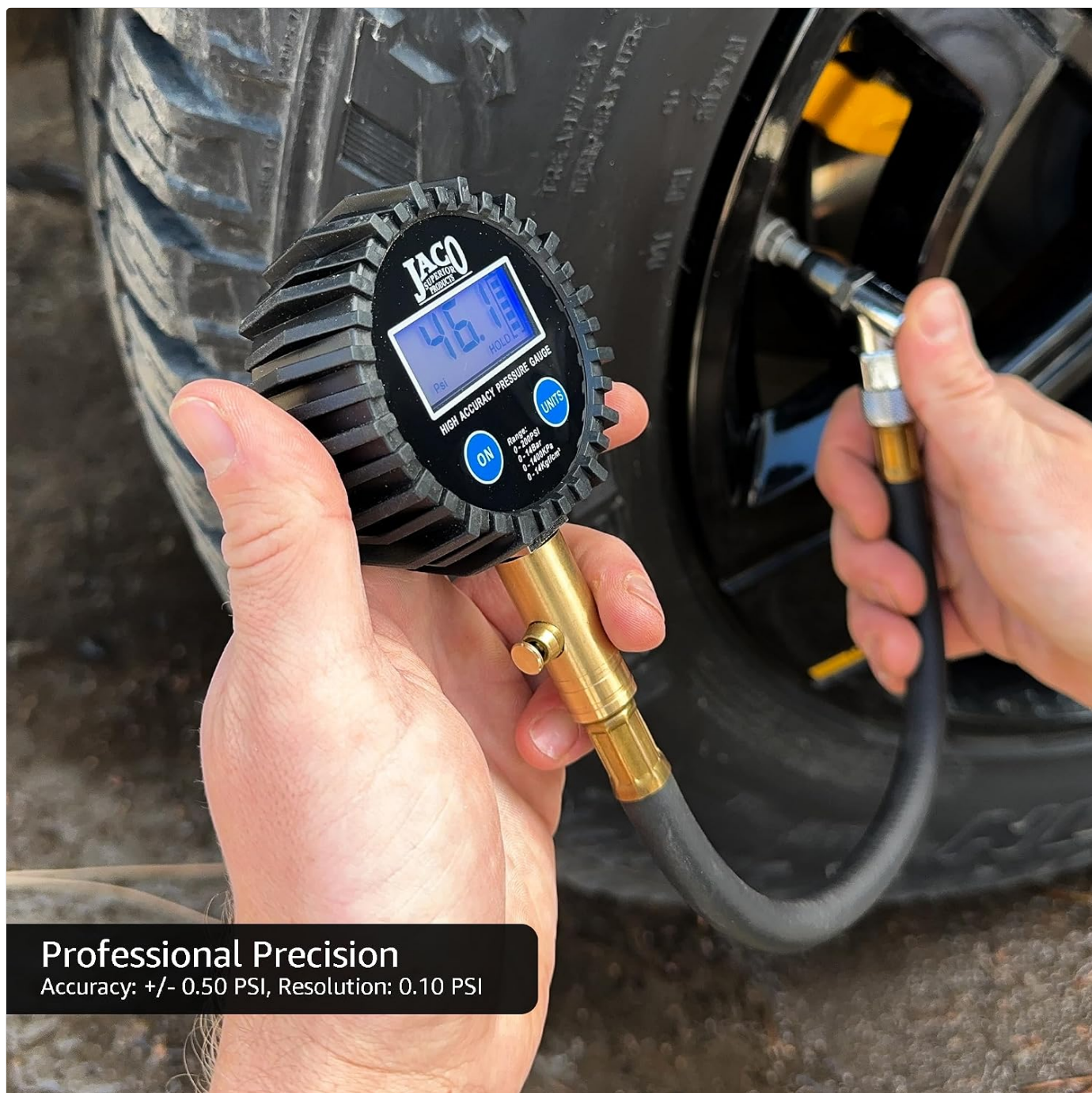
Figure 3: Measuring tire pressure with professional precision.
