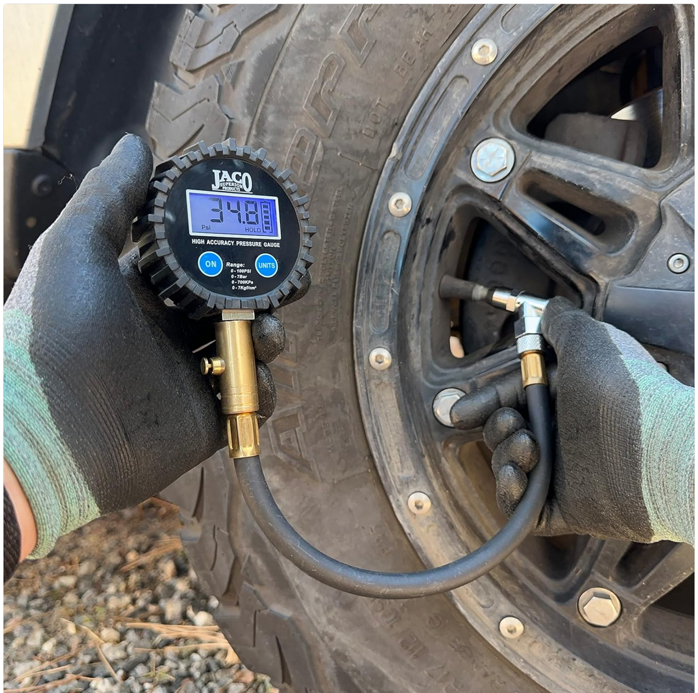
Figure 5: Deflating a tire using the bleeder valve.
