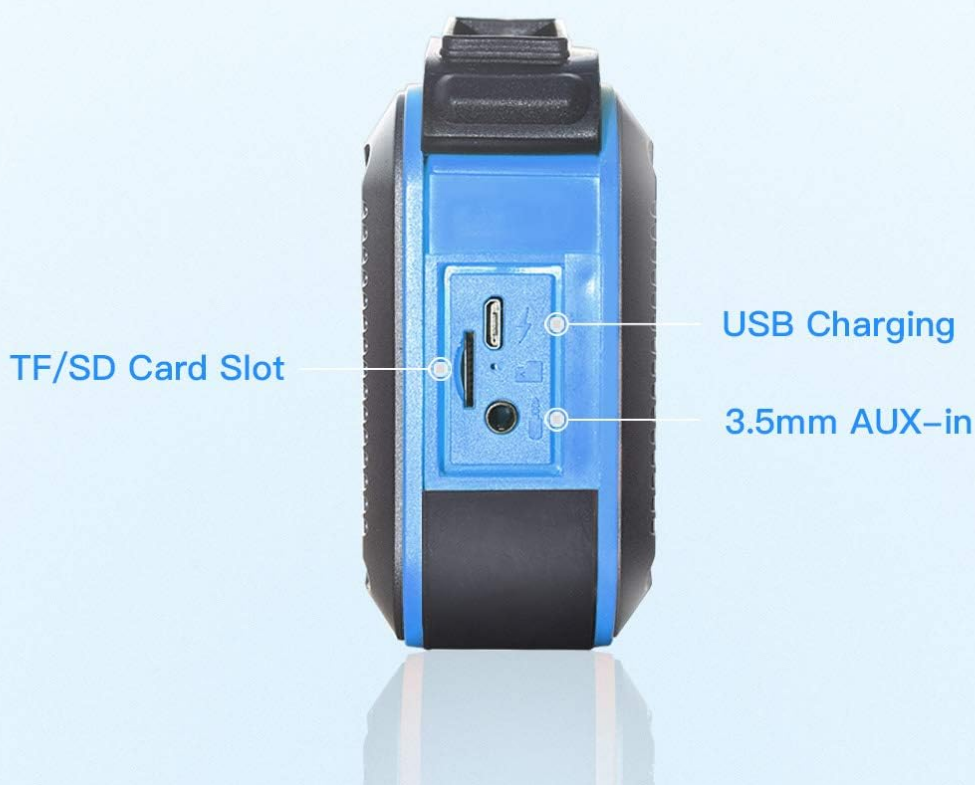
Figure 5: Multi-functional playback ports including USB charging, TF/SD card slot, and AUX-in.
