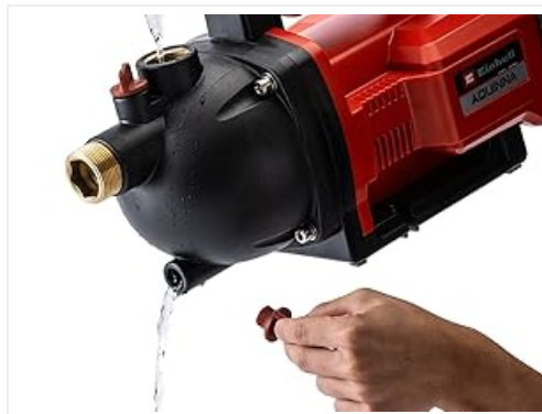
Figure 12: Draining the Pump. A visual guide to opening the drain screw to remove water from the pump for winter storage.
