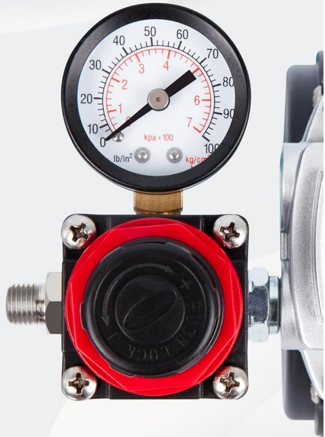
Figure 4.3: Air Pressure Regulator. This component allows for precise adjustment of the output air pressure using the knob control. The integrated gauge displays the current pressure in both PSI and Bar. To adjust, pull the knob up and rotate, then push down to lock.
