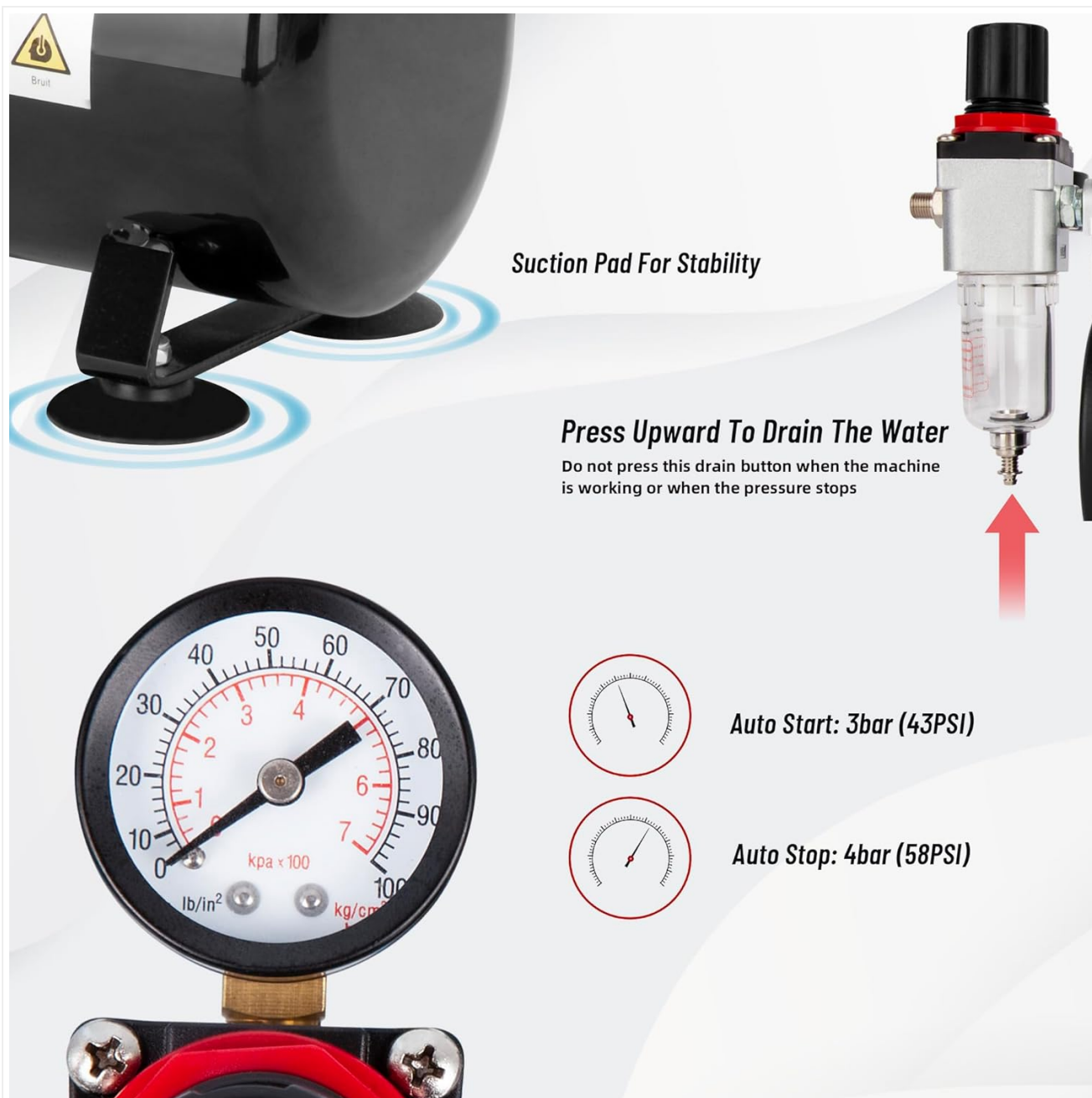
Figure 4.4: Additional features. This image shows the suction pads for stability during operation, the auto start (3 Bar / 43 PSI) and auto stop (4 Bar / 58 PSI) pressure settings, and the drain button for releasing accumulated water from the moisture trap.
