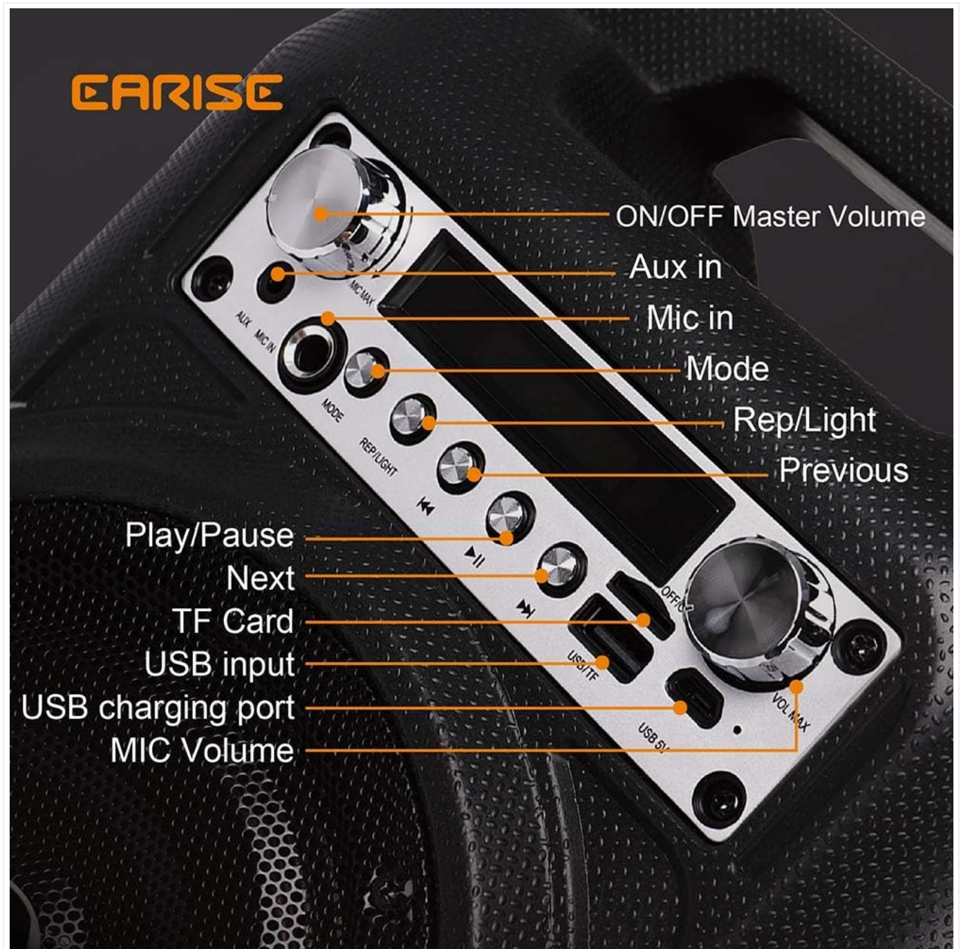
Image: Close-up view of the EARISE T35 control panel, indicating the function of each button and knob.
