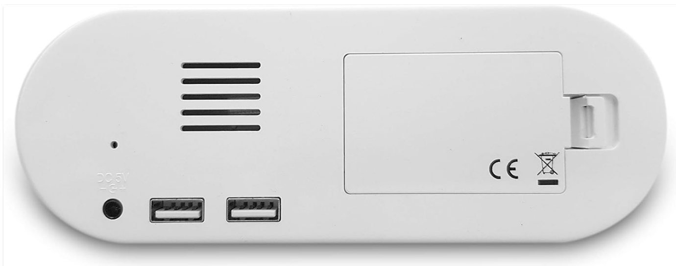
Image: Rear view of the alarm clock, showing the DC 5V power input, two USB charging ports, and the cover for the battery backup compartment.
