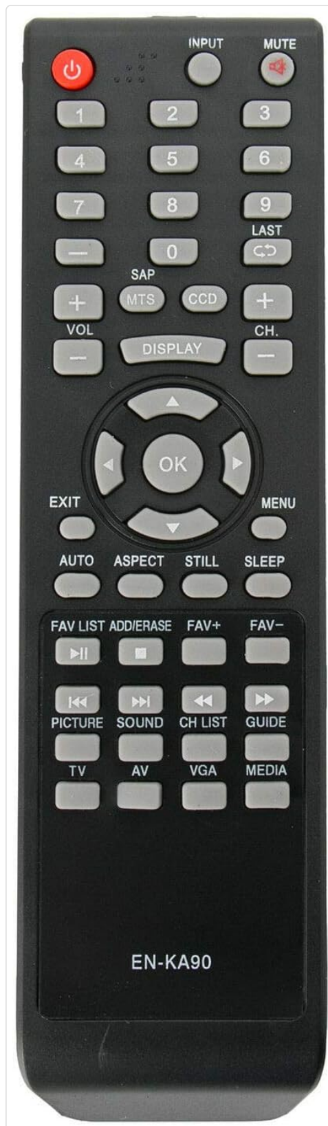
Image: Front view of the UBay EN-KA90 remote control, showing all buttons and their labels. The remote is black with grey buttons. Key buttons include Power, Input, Mute, Number Pad, Volume Up/Down, Channel Up/Down, Navigation Pad with OK, Menu, Exit, and various function buttons like Auto, Aspect, Still, Sleep, FAV List, Picture, Sound, CH List, Guide, TV, AV, VGA, and Media.
