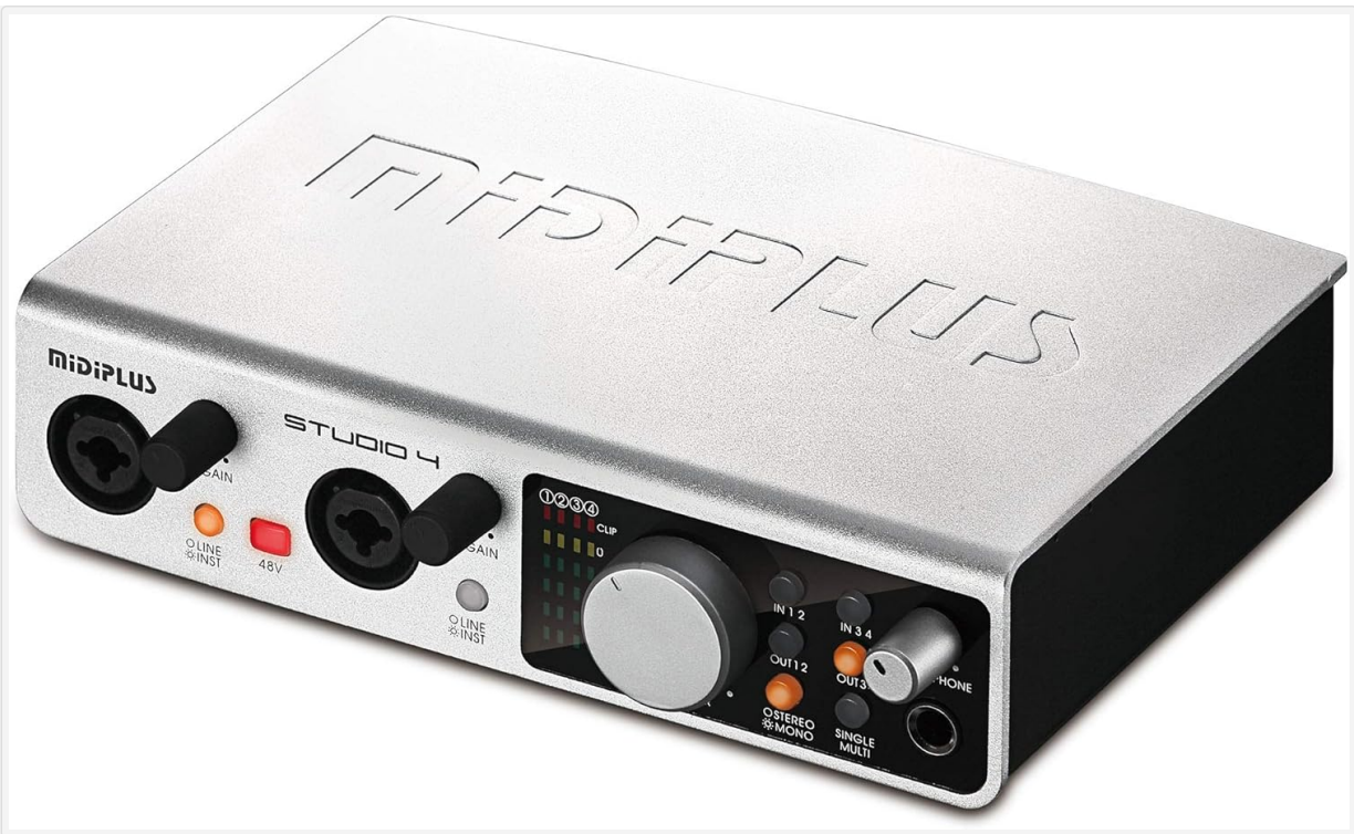
Figure 1: Front view of the Midiplus Studio 4 Audio Interface, showing inputs, gain knobs, and monitoring controls.
