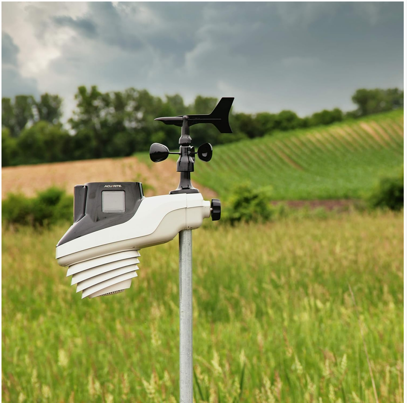
Figure 2: The AcuRite Atlas Weather Sensor mounted on a pole in an open area, demonstrating ideal placement for unobstructed readings.
