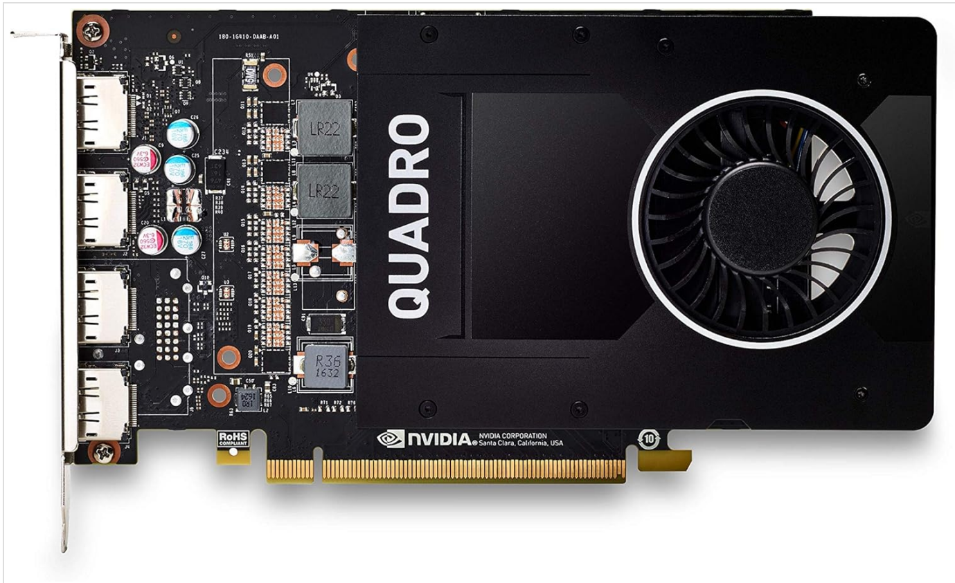
Figure 2.2: Top view of the NVIDIA Quadro P2200 Graphics Card, highlighting the Quadro branding and fan shroud.
