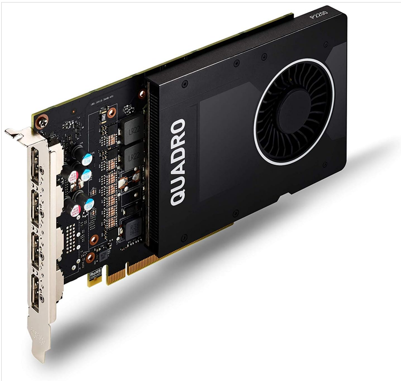
Figure 2.3: Side view of the NVIDIA Quadro P2200 Graphics Card, showing the PCIe connector and overall length.
