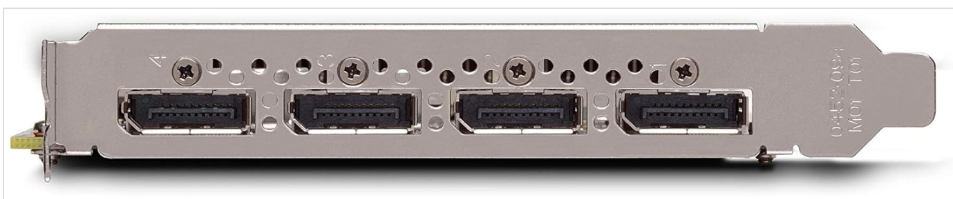
Figure 2.4: Rear view of the NVIDIA Quadro P2200 Graphics Card, displaying the four DisplayPort outputs.
