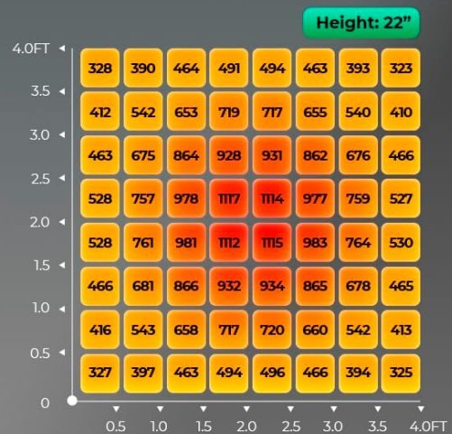
Image: A PPFD (Photosynthetic Photon Flux Density) map for the TS 3000, showing light intensity distribution at 12, 18, and 22 inches height within a 4x4ft grow tent.
