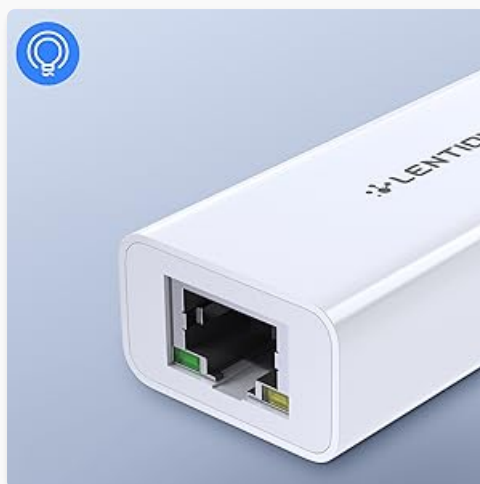
Image 3.1: Close-up view of the RJ45 port on the adapter, showing the green and yellow LED indicators for connection and activity.
