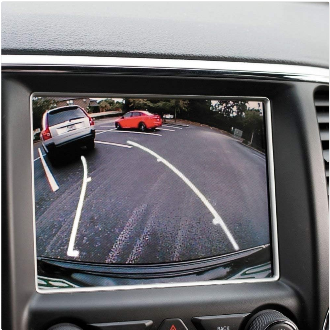
Image: An in-car display showing the backup camera's view. The screen displays a wide-angle image of the rear environment, complete with dynamic parking guidelines overlaid on the video feed.
