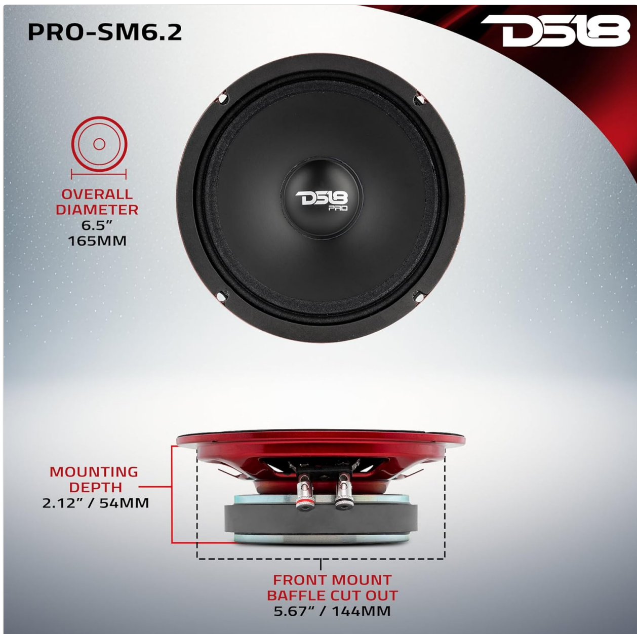
Figure 3: Detailed dimensions for the DS18 PRO-SM6.2 loudspeaker, including overall diameter, mounting depth, and cut-out
