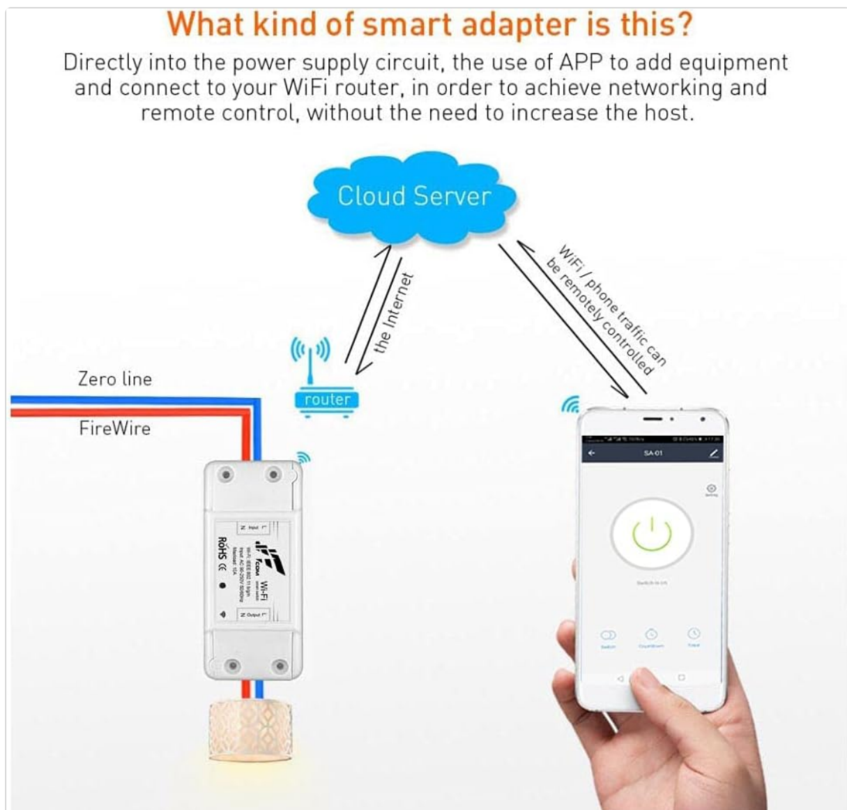
Figure 4: Conceptual diagram illustrating the smart switch's connection to a router and remote control via a smartphone application.
