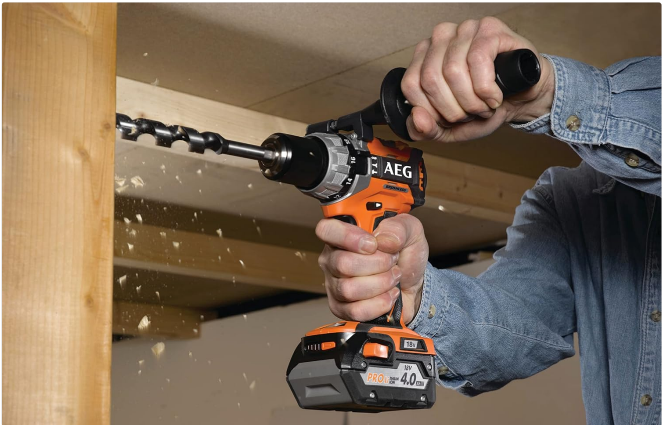
Figure 2: Detailed view of the hammer drill, showing the adjustable side handle, chuck, and battery connection point.
