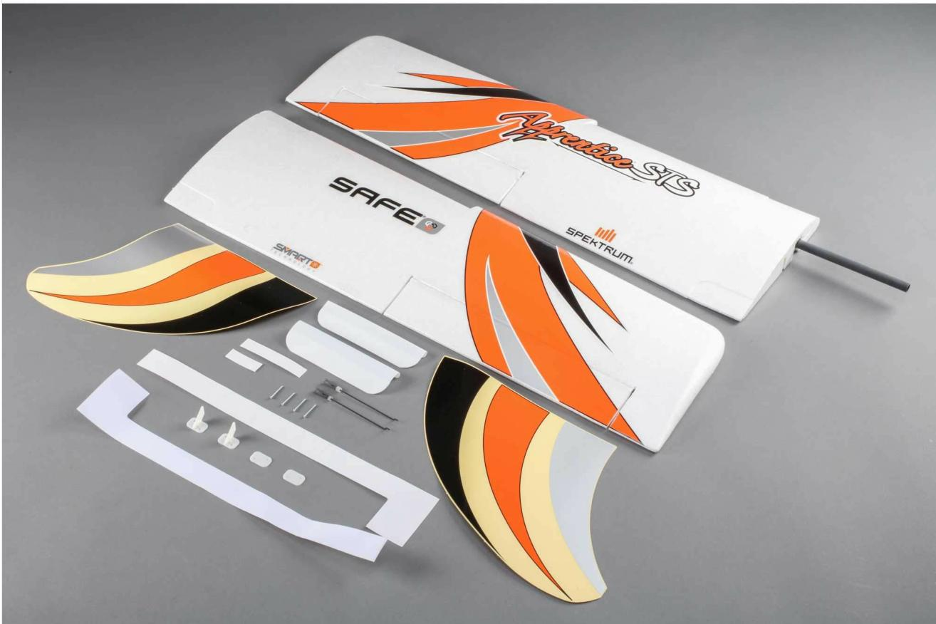
Image: The E-flite Apprentice STS Replacement Wing Set, showing the two main wing sections, various small plastic parts, control rods, and decal sheets.
