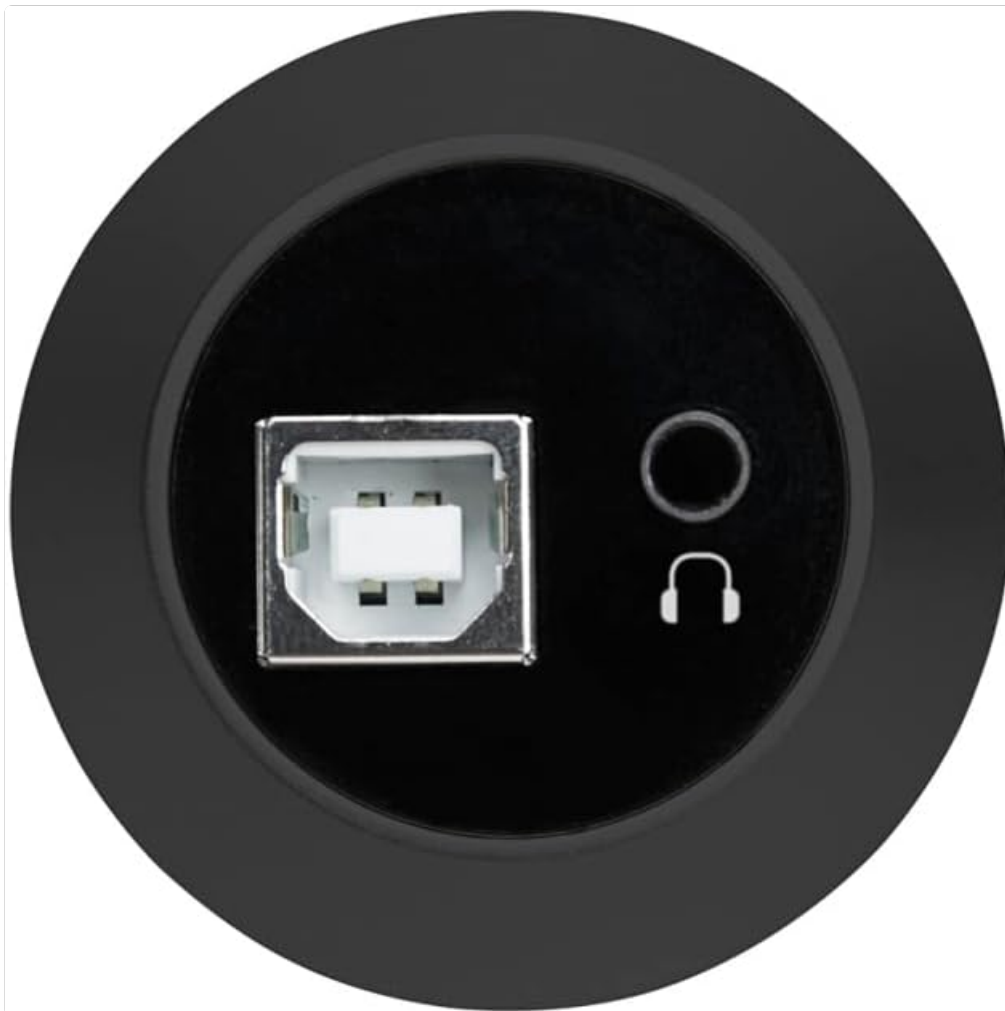
Image 4.1: USB Type B and 3.5mm Headphone Ports.
