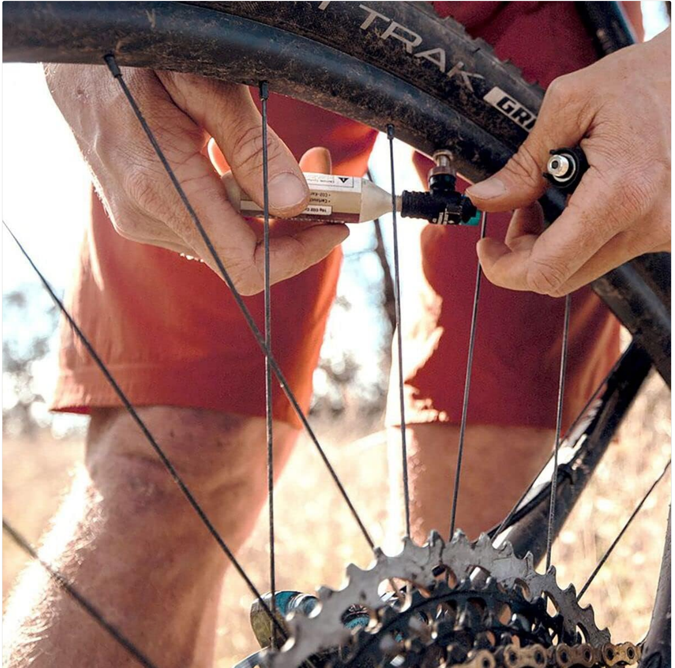
Figure 4: A user demonstrating the insertion of a tire plug into a punctured bicycle tire using the Blackburn Pro Plugger tool.
