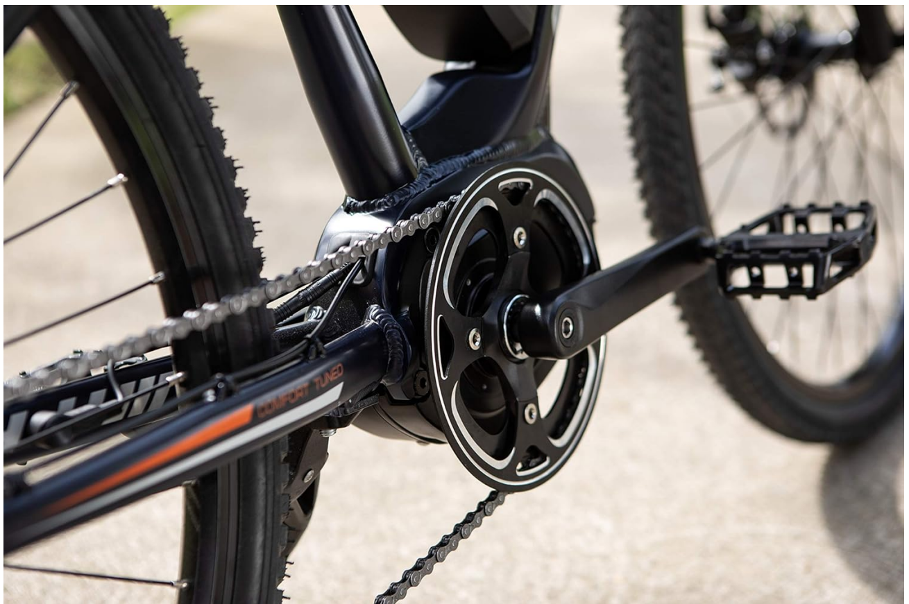
Figure 3.3: Mid-Drive Motor. A detailed view of the 250-watt mid-drive motor integrated into the bike's frame, connected to the crankset and chain.
