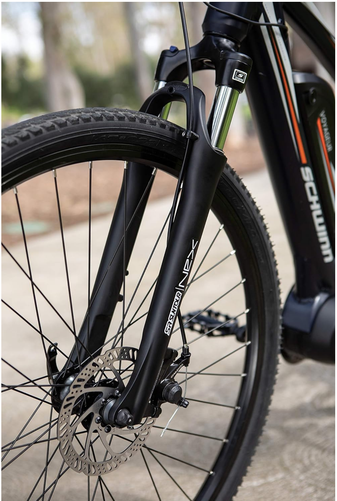
Figure 3.5: Front Suspension and Disc Brake. A close-up view of the SR Suntour NEX suspension fork and the mechanical disc brake caliper and rotor on the front wheel.
