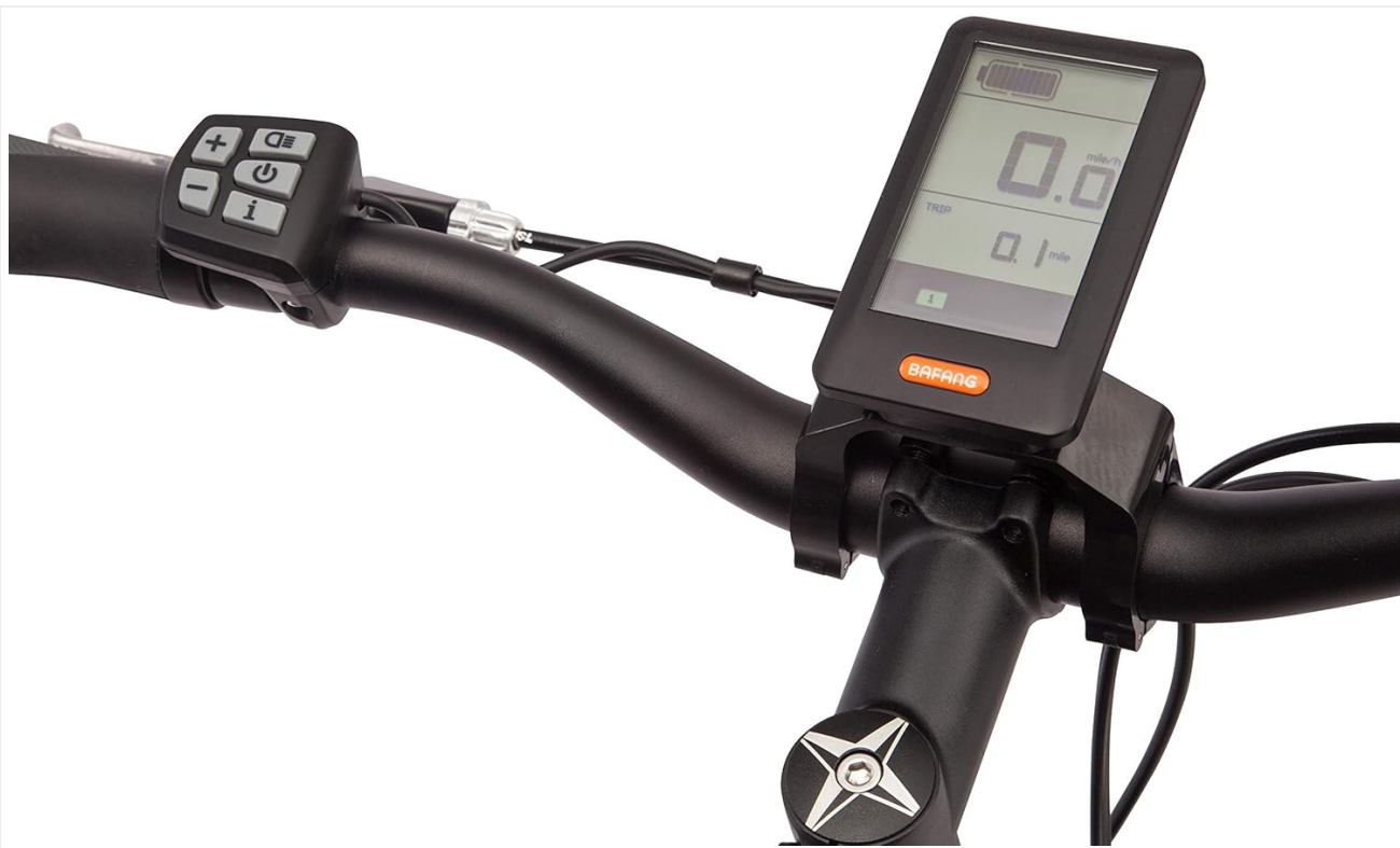
Figure 5.2: Detailed View of Display and Controller. A closer look at the Bafang LCD display and the control unit, illustrating the interface for managing pedal assist levels and viewing ride data.
