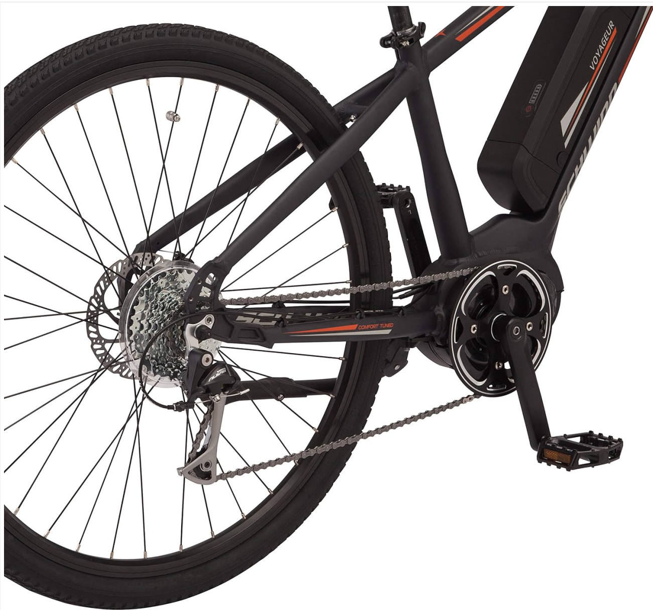
Figure 3.7: Rear Drivetrain. This image details the rear wheel's cassette, chain, and Shimano derailleur, part of the 8-speed drivetrain.
