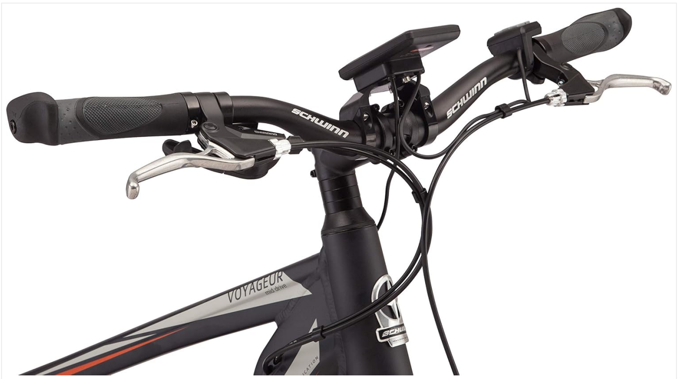
Figure 3.2: Handlebar Assembly. This image shows the handlebars, brake levers, gear shifters, and the mounting point for the LCD display and controller.
