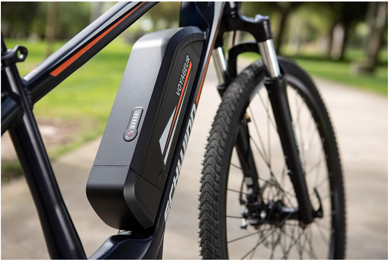
Figure 3.4: Integrated Battery Pack. This image shows the removable battery pack, labeled 'Voyageur', integrated into the downtube of the bicycle frame, with its charge indicator visible.
