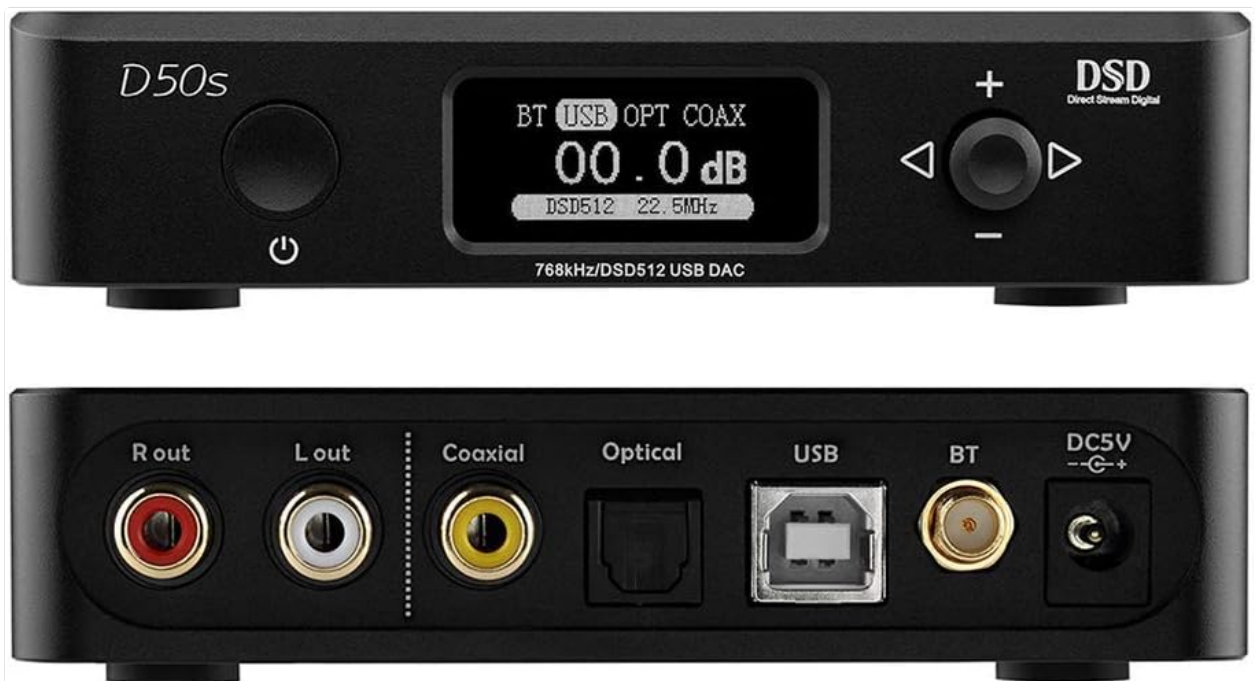
Image 2.2.2: Front and Rear Panels of TOPPING D50s. This image provides a comprehensive view of both the front panel with its display and controls, and the rear panel detailing all available input and output connections, including RCA outputs, Coaxial, Optical, USB, Bluetooth antenna port, and DC 5V power input.
