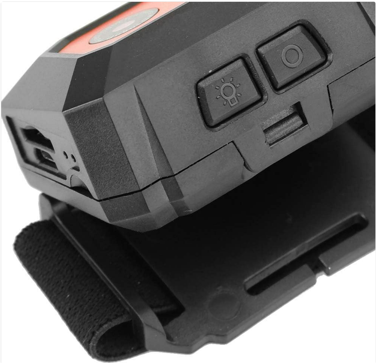
Image 5.2: A side view of the camera, illustrating the placement of control buttons and the Mini USB port for charging and data transfer.
