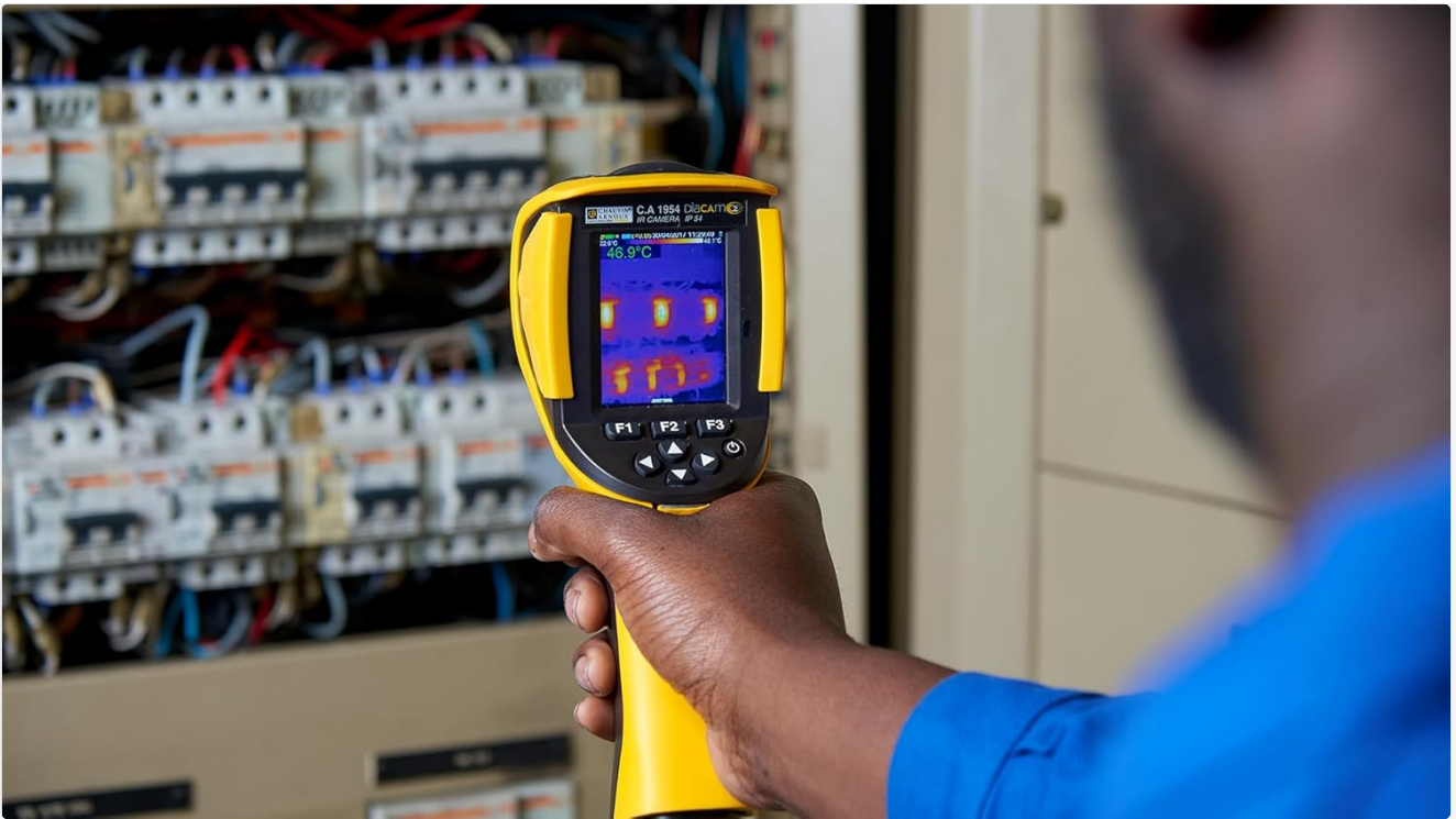
Figure 3: A user operating the C.A 1954 thermal camera to inspect an electrical panel.
