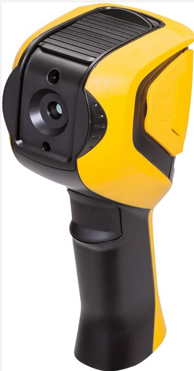
Figure 4: Rear view of the C.A 1954, showing the lens and its protective sliding shutter.
