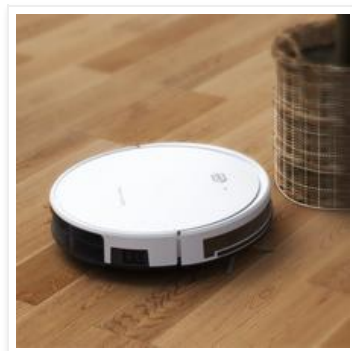
Image: Anti-collision sensors help the robot avoid obstacles and protect furniture.
