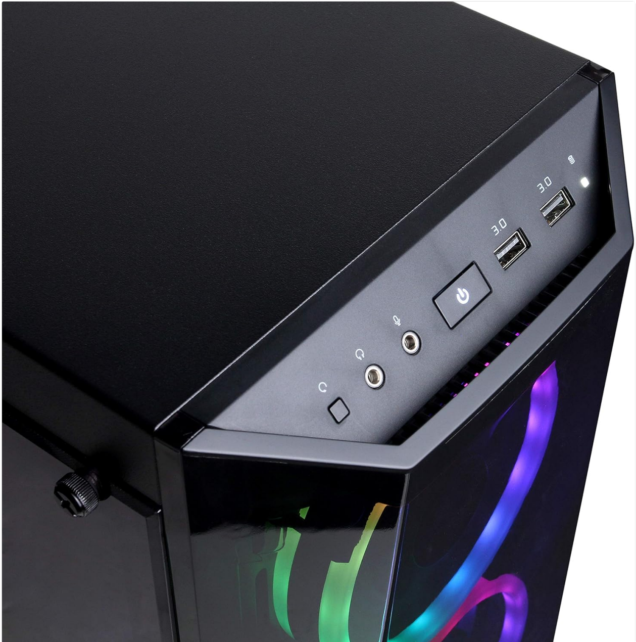
Image 3.1: Top panel of the PC showing the power button, USB 3.0 ports, and audio jacks.
