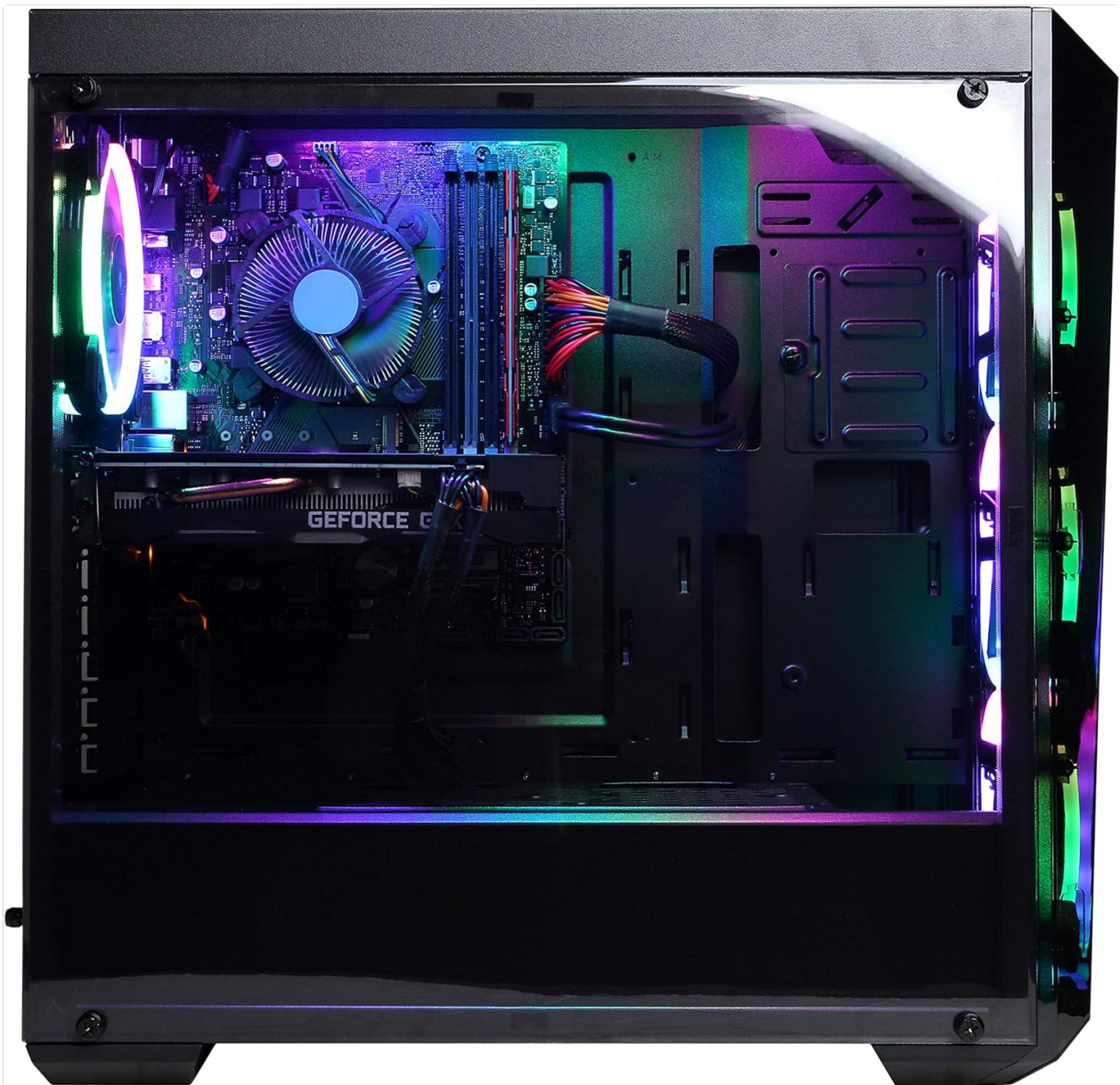
Image 3.2: Internal view of the PC showcasing the motherboard, CPU cooler, RAM, and graphics card.
