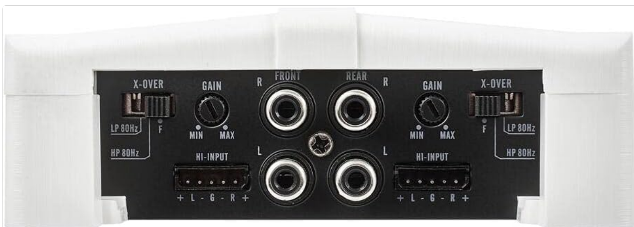
Figure 3: Rear panel of the Power Acoustik MSA4-1300D amplifier, showing RCA inputs, High-Input terminals, Gain controls, and X-OVER (crossover) switches for both front and rear channels.
