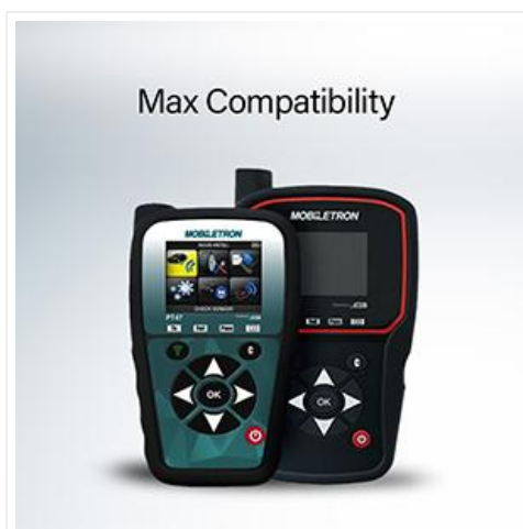
Image 3.2: Mobiletron PT47 and other compatible programmers for sensor configuration.
