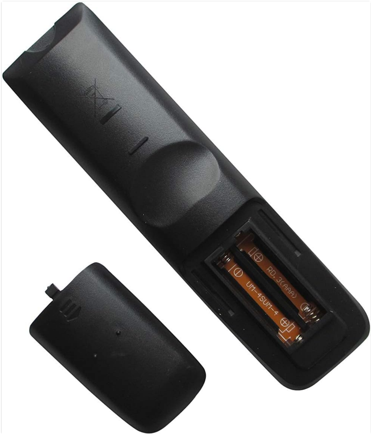
Figure 1: Rear view of the remote control with the battery cover removed, illustrating the correct orientation for AAA battery insertion.
