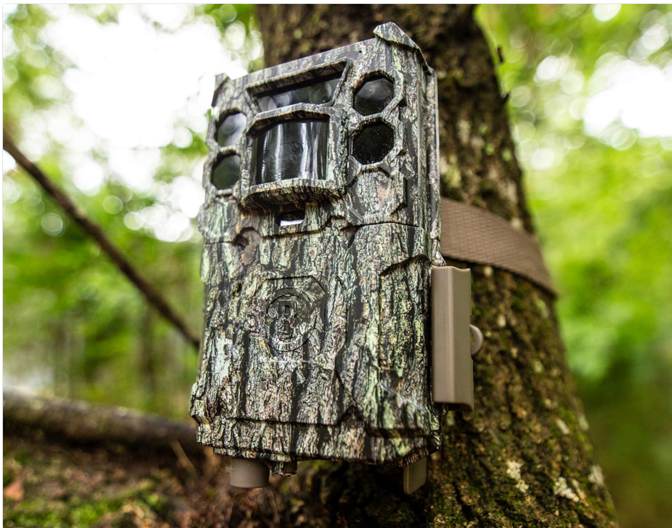
Figure 3.3: The trail camera securely mounted to a tree using the provided strap.
