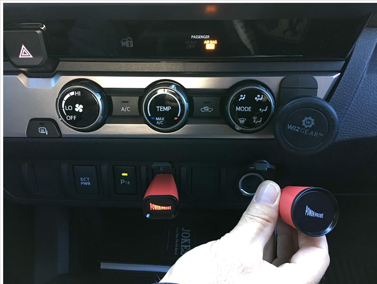
Figure 5.1: The Power Probe Mini Probe TST12V inserted into a vehicle's 12V outlet for testing.
