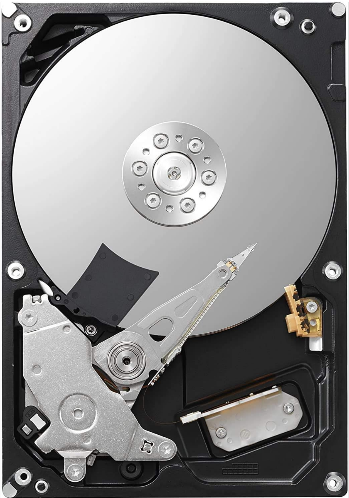
Image: Top-down view of the internal components of the Toshiba P300 hard drive, showing the platter and read/write head.
