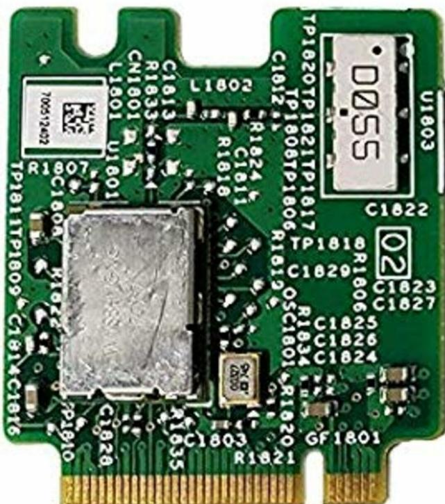
Image 1: Avaya J100 Wireless Module. This image displays the compact design of the module, showing its connectors and casing.
