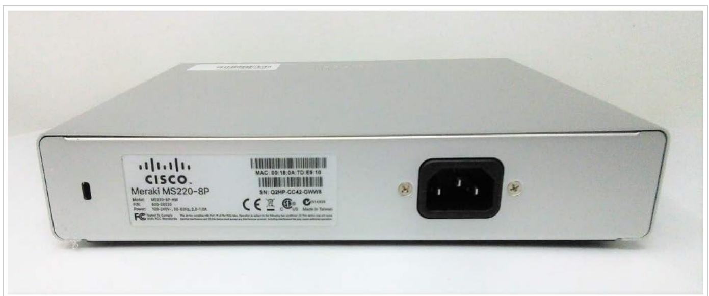
Figure 2: Rear view of the Cisco Meraki MS220-8P-HW switch. This image shows the AC power input socket on the right. On the left, a product label provides essential information including the Cisco Meraki logo, Model: MS220-8P-HW, Part No: 600-38109, Power specifications (100-240V, 50-60Hz, 2.0-1.0A), MAC address, and Serial Number (SN: Q2HP-CC4J-QWWR).
